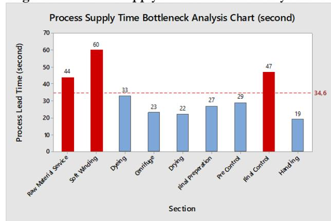
Accordingly, considering the durations of the operation steps, the following bottleneck analysis was carried out for the operations and the bottlenecks were determined as shown in Fig. 14 in order to create continuous flow. The value stream map team prepared the future situation map given in Figure 16 in accordance with the above findings.
