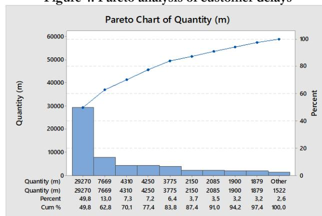
For this purpose, it is aimed to improve the customer delays originating from the dyeing department included in the pareto analysis with the MG01 code, which is the half of the total delays and decided to create a value stream map in this section. It was started by analyzing the production carried out in the operation, by interviewing the engineers who planned and controlling the production. Information about procurement, stock, production processes and employees was obtained.
